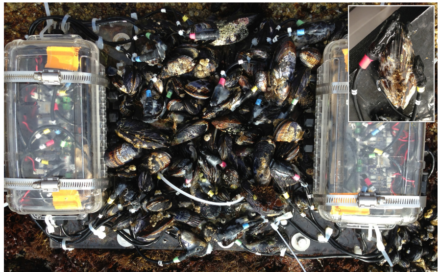
FIGURE 1 Overhead view of the experimental mussel bed comprising 12 instrumented individuals of Mytilus californianus and additional live mussels. Inset: close-up of an instrumented mussel showing the gape sensor (posterior end, top of photo), accelerometer/magnetometer (right valve), and thermocouple (small black wire leading to ventral midpoint of the left valve)
